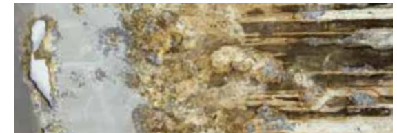
Unprotected coil that's been in contact with ACQ lumber. Conditions simulated in a 60 day laboratory test.
